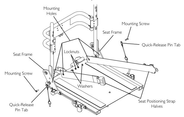
FIGURE 8.2 Replacing Seat Positioning Strap
